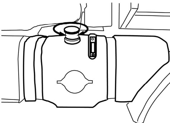
The **320** litre diesel oil tank is located on the right-hand side. Before filling the tank, you must :
