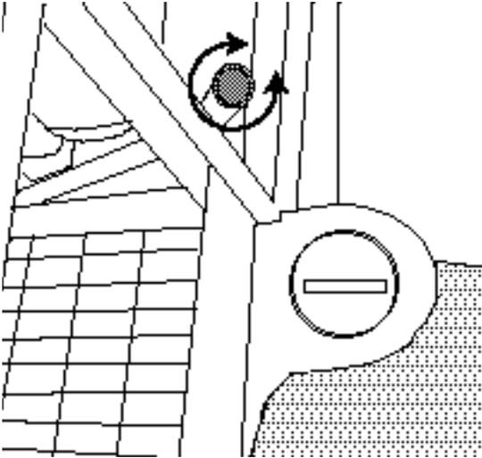
This **60** litre reservoir is located under the cab. The filler cap is situated on the reservoir on the left-hand side of the machine **(1)**
