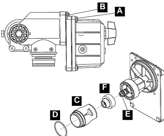
If it becomes difficult to build up sufficient pressure or if pressure fluctuations occur, it may be necessary to renew cone and cylinder. A Hardi kit is available for this purpose n°. 741293
