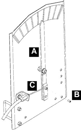
If the position of the pointer on the indicator does not correspond to the actual boom position, the pointer **(A)** can be adjusted.
