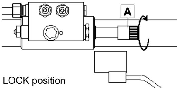
In case of power failure the pendulum device can be locked as follows :
