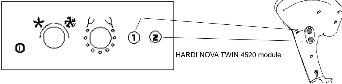
By pressing the TWIN module pre-set or switches on the joystick for more than 3 seconds , the current settings of the fan speed and the air slot angle is memorized.
