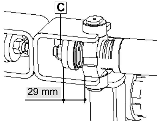
**Adjustment of Pendulum device**
