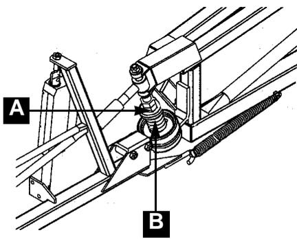
The breakaway section must be released when a force of approximately 150 N (34 lb) is applied to the extremity of the breakaway section. If necessary break-away section is adjusted as follows :
