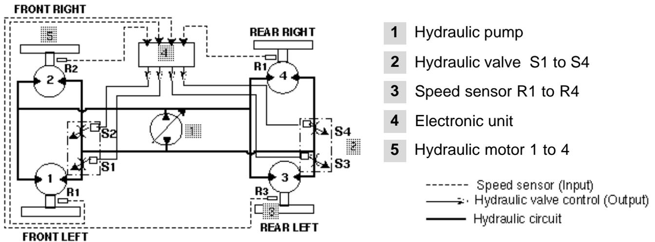
The speed sensors **R1** to **R4** incorporated the hydraulic motors **(5)** continuously measure the rotation speed of each drive wheel. The regulating computer **(4)** compares those speeds and if necessary reduces hydraulic flow to the wheel which has a tendency to spin.
