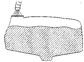
**WARNING: Do not let filling hose etc. enter the tank. Keep it outside the tank, pointing towards the filling**
