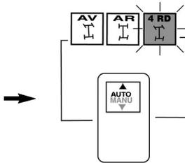
When the wheels are turned, the red warning lamp goes out but green warning lamp is still activated..
