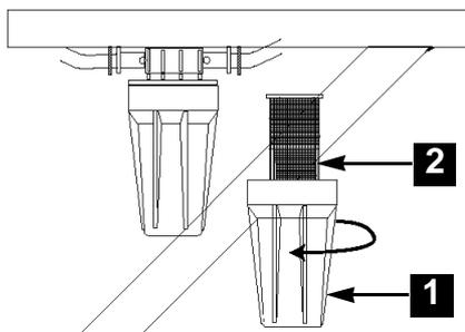
\* blue filter 300 microns (50 mesh), delivery as standard
