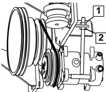
Check the tension of the air conditioning belt, for this purpose :
