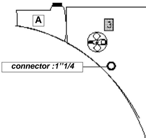
Connect a pipe to connector and open valve **(3)** to fill the rinsing tank.
