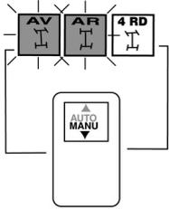
In this operating mode an adapted crab steer can be done by using the steering wheel and pedal.
