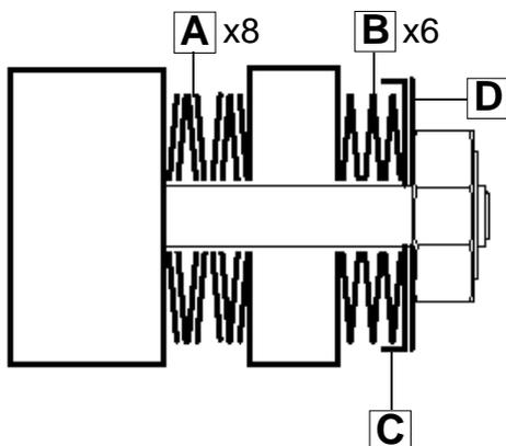
5. Place new spring washers respecting the right position as shown on the picture :
