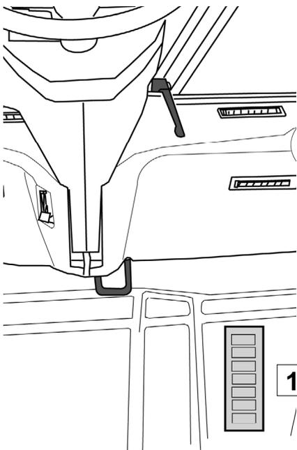
On some models, the sprayer is fitted with a combined emergency and parking brake, which can be variable proportioned. On this model, the operating pedal (1) is placed on the floor.
