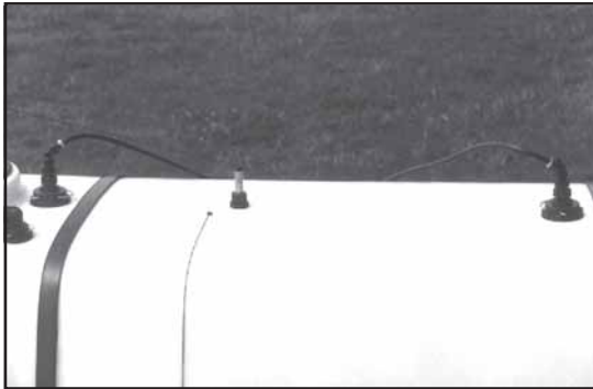
Fig. 39 Rinse Nozzle on Top of Tank
