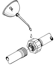
The O-ring is lubricated **ALL THE WAY ROUND** before fitting on to the nozzle tube. Use non-mineral lubricant.
