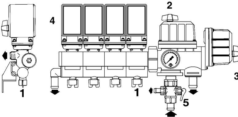
1. Adjustment screw for pressure equalization
