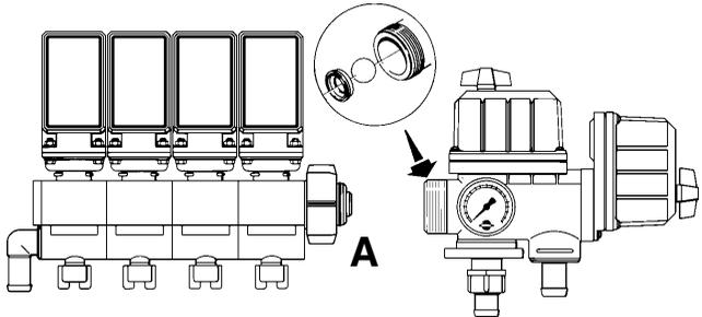
Check the ball for sharp edges and scratches, and check the ball seat for cracks and wear - replace if necessary.
