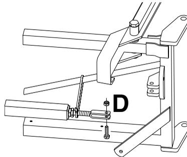
6. Fit the activating rod again, fold the boom, and check the spring compression again. If necessary, carry out point 5 again.
