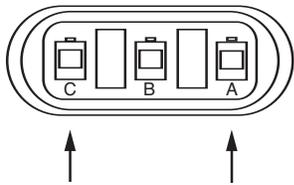
**REMOTE RUN/HOLD INPUT:** Disconnect the remote run/hold sensor (or jumper cover) from the main harness.
