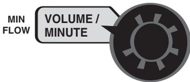
For example: If the minimum flow rate for the nozzle you are using is .22 GPM at their minimum recommended pressure and your boom has 20 nozzles, enter 4.4 as the MIN FLOW value (.22 x 20 = 4.4). The system **WILL NOT** apply at a rate lower than this value when spraying in AUTO. This value should be checked/ changed for each different nozzle that you use.
