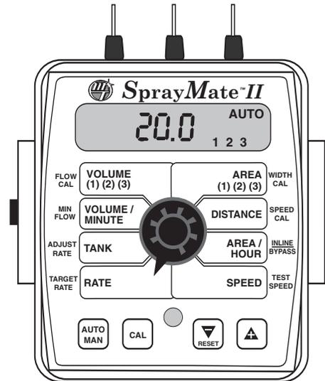
During normal operation, when manual “MAN” control mode is active and the Run/Hold switch is in the RUN position, pressing the “+” or “-” buttons will increase or decrease the application rate by opening or closing the servo valve (control valve).
