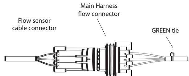
Connect flow sensor cable to green-tie console cable.
