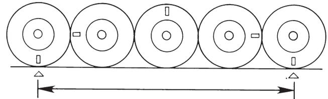
To determine SPEED CAL, measure the distance of one complete wheel revolution and divide by the number of magnets installed.
