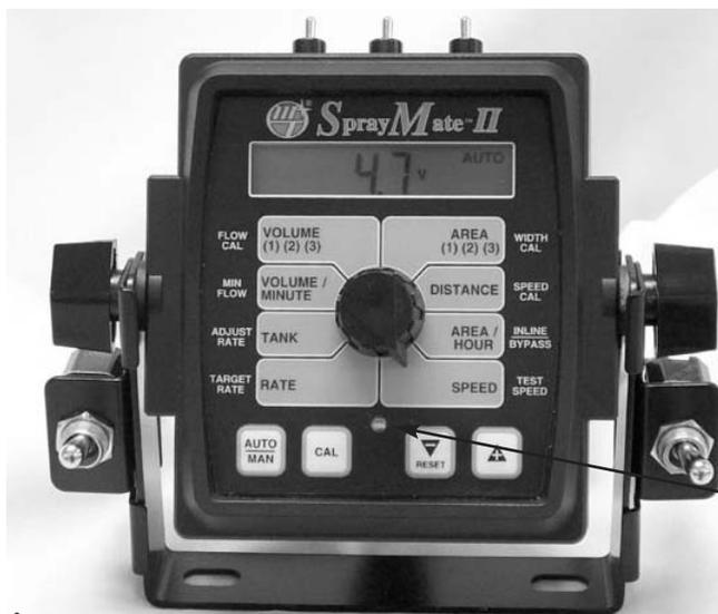
**WARNING LIGHT:** Indicates over or under application of 10% of the Target Rate. Also lit when in CAL.
