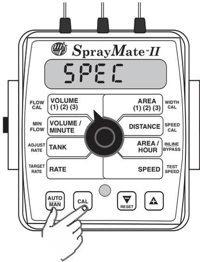
Turn the rotary switch to the AREA/HOUR position and use the "+" or "-" button to choose NH3. While in Special Calibration mode, other parameters can also be adjusted, see Special Calibration section on pages 27-28. NOTE: to save the values you changed, you MUST exit Calibration by pressing the CAL button for one second.
