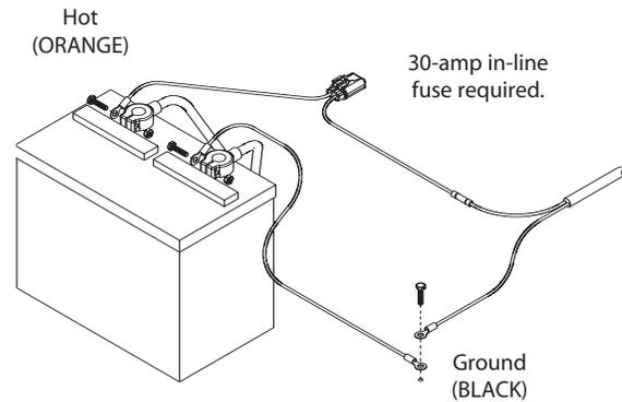
**NOTE: be sure to route cables away from sharp edges, areas of high heat and moving parts. Secure all cables firmly with plastic cable ties.**
