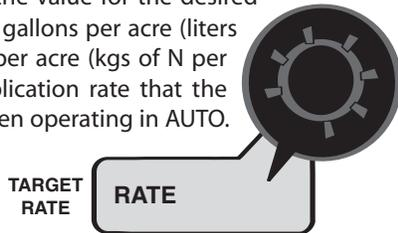
**ADJUST RATE:** Enter the value for the desired amount of change in gallons per acre (liters per hectare) to be used for making on-the-go rate adjustments when operating in AUTO. For example, if a value "1.0" is entered, you will be able to increase or decrease your application rate in one-gallon (liter) or lb. (kg) increments during operation in AUTO. To disable this feature, simply enter ".0" for a value.
