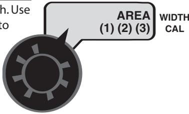
**SETTING TOOL BAR WIDTH:** In order to accurately measure the pounds (kg) of "N" applied per acre (hectare), it is important to determine the correct "working" width. The "working" width is the width of ground being affected by any operation. This should be measured to the nearest inch (millimeter).
