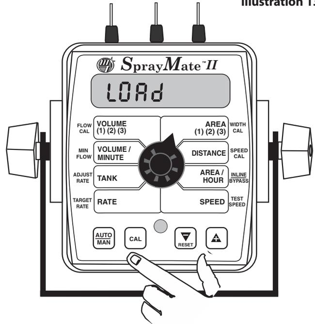
**NOTE: In metric, the width will have a decimal point, in English there is no decimal point. Also, changing from English to Metric mode may change or alter any previously entered calibration values. After switching measurement modes, confirm that all calibration values are correct.**
