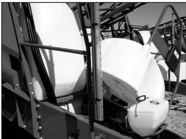
Working Platform tilted for access
