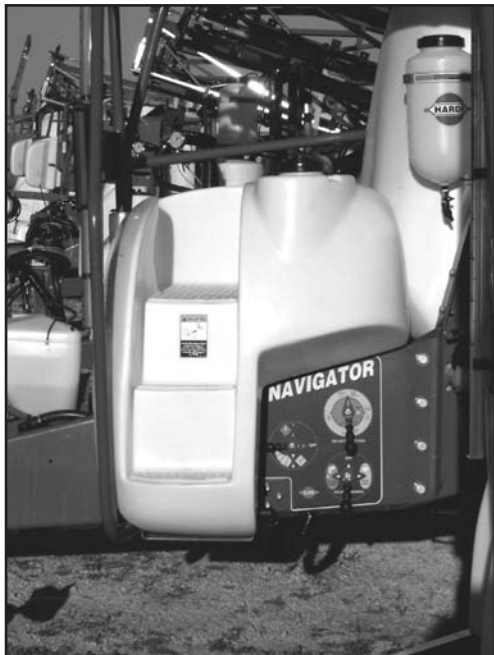
Working Platform / Flush Tank
