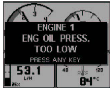
Figure 7.8.1: A representative alarm pop-up message, showing low engine oil pressure.
