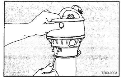
2. Remove the nylon bearing and pull off the protection tube.
