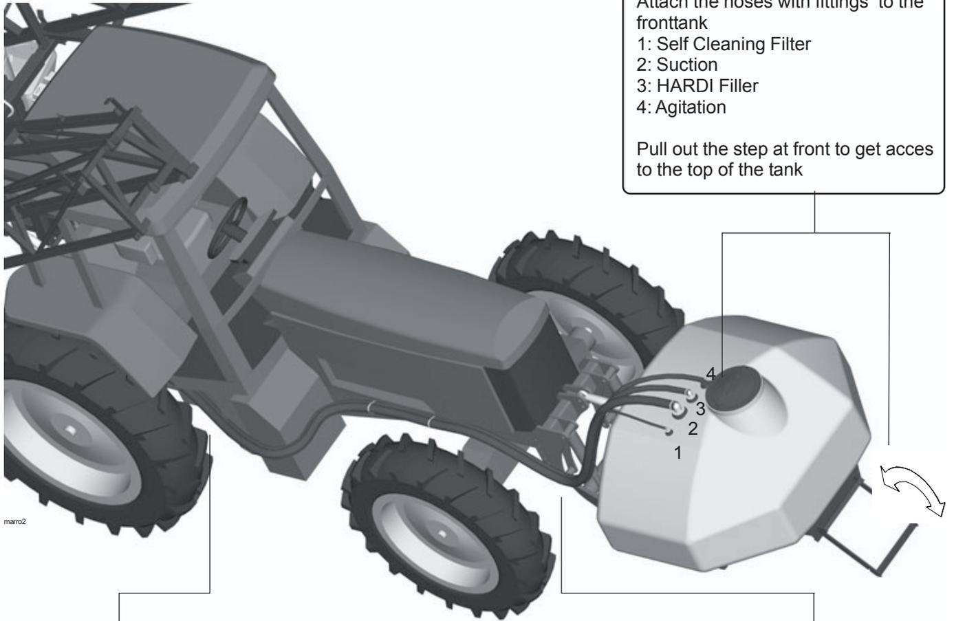
The hoses are led from the MANI-FOLD valves along the side of the tractor to the front tank as shown on the drawing. Routing of hoses will vary depending on tractor model.
