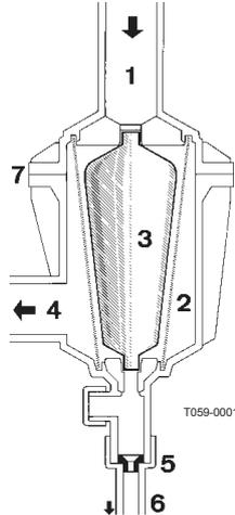
**IMPORTANT!** The ball valve underneath the self-cleaning filter should normally be open, but must be closed in the following cases:
