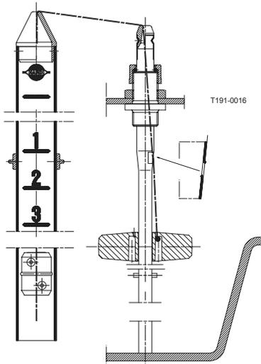
4. Check cord and valve flap assembly **C** for wear, replace seal **D** and assemble again.
