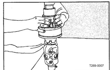
6. Check alignment and locking of the tabs by tapping the universal cross cover lightly.
