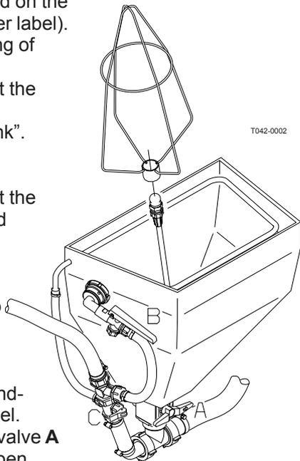
**WARNING!** Do not press lever **B** unless the multi-hole nozzle is covered by a container to avoid spray liquid hitting the operator.
