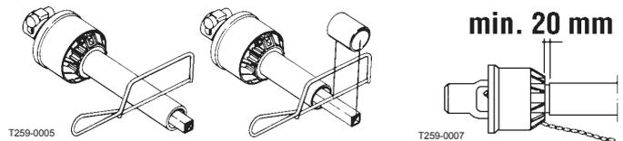
4. The two parts are shortened equally. Use a saw, and file the profiles afterwards to remove burrs.
