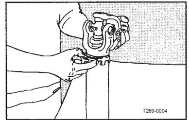
3. Grease protection tube bearing groove on the inner yoke.
