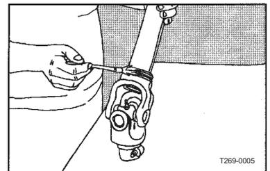
4. Slide on the shield tube and fit the bearings tabs into the slots.
