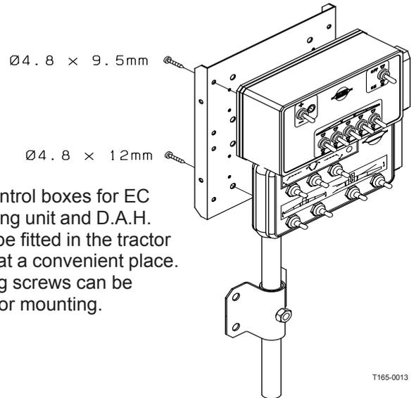
The control boxes for EC operating unit and D.A.H. are to be fitted in the tractor cabin at a convenient place. Tapping screws can be used for mounting.
