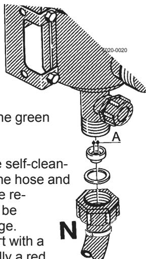
When cleaning the filter remove hose **N** and the hose at the safety valve, and check there are no residues.
