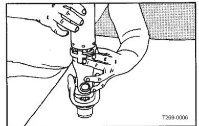
5. Slide the universal cross cover over the protection tube and align the grease nipple with the grease channel on the bearing. Press the universal cross cover onto the tabs until they lock.
