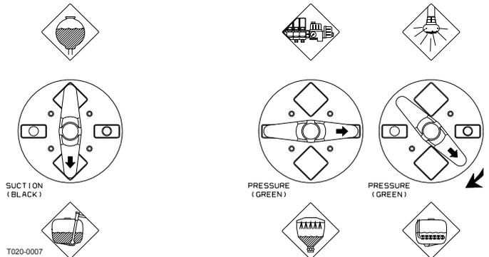
13. When the spray liquid is well mixed, turn handle on the Pressure Manifold towards "Spraying" position. Keep P.T.O. engaged so the spray liquid is continuously agitated until it has been sprayed on the crop.
