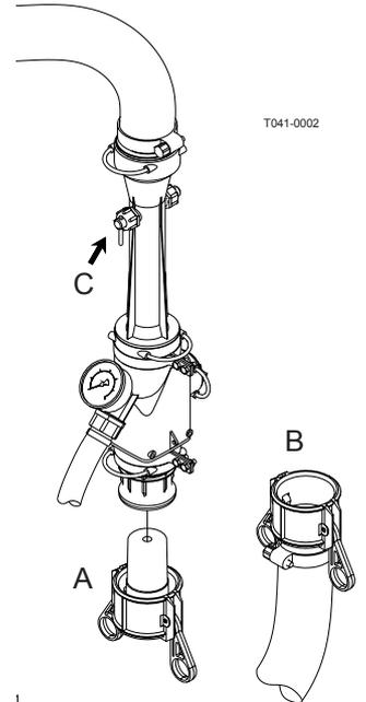
**NOTE:** Turn handle towards EC-operating unit **before** turning away from Fast Filler in order to avoid peak pressure blowing the safety valve!
