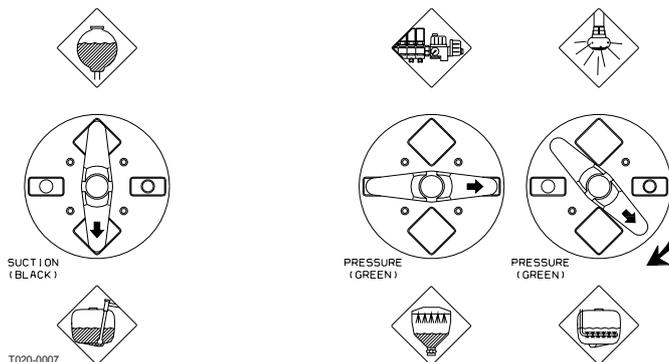
12. When the spray liquid is well mixed, turn handle on the Pressure Manifold towards "Spraying" position. Keep P.T.O. engaged so the spray liquid is continuously agitated until it has been sprayed on the crop.
