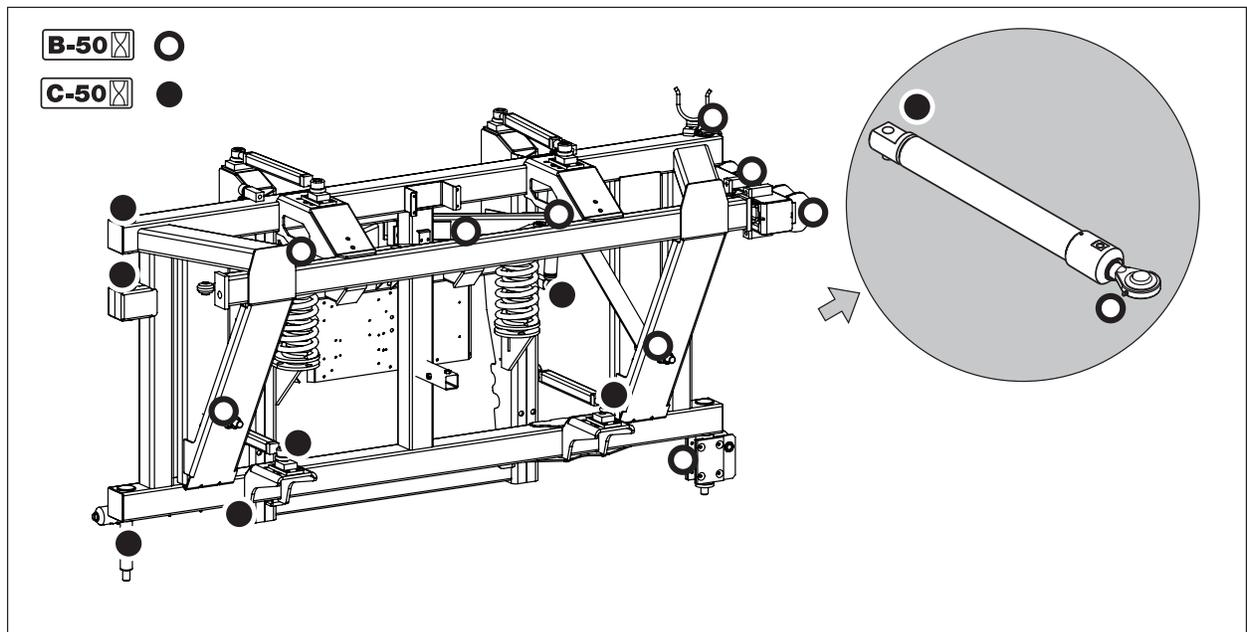
Boom lubrication & oiling plan (118')
