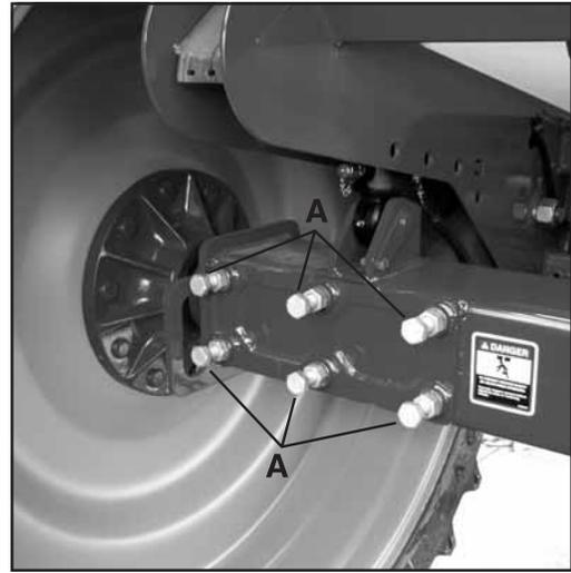
See "50 hours service - Wheel bolts and nuts" in the "Maintenance" section for proper torque and tightening sequence of wheel hubs to rims.
