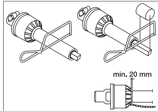
7. Fit the chains to prevent the protection guards from rotating with the shaft.
