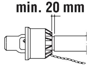
It is important for the personal safety of the operator that the transmission shaft is intact. The protection guards must cover the whole shaft. This includes the universal cross covers at each end of the shaft. The chains are connected so that the protection guards do not rotate with the shaft.
