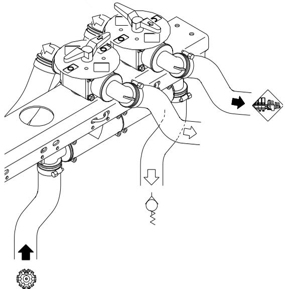
If all the green pressure valves are closed the safety valve will open inside the tank.
