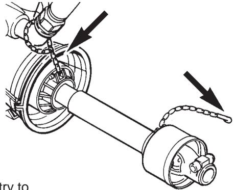
To ensure long life of the shaft, try to avoid working angles greater than 15°. For the same reason the pump is situated at the back of the tank frame. This permits a longer transmission shaft and thereby less angling of the cross journal when altering the position of the sprayer with the tractor lift arms.
