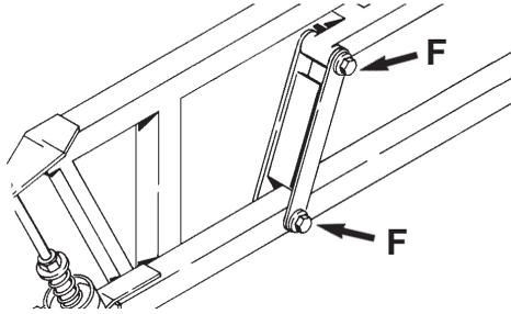
Adjust trapeze bolts **F** so it is not tight nor loose. Minor adjustment in the field may be necessary.
