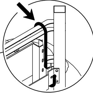
**WARNING:** Always secure the boom before servicing the pump.
