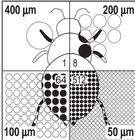
Halving one 400 mm drop produces 8 drops of 200 μm. With these smaller drops, it is possible to cover about twice the area.
