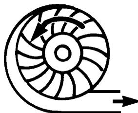
The blower housing may direct the air out to both sides or to one side.
