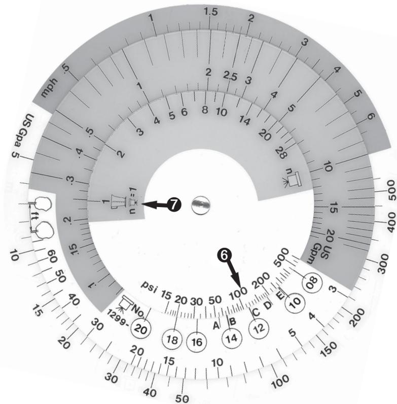
Align the nozzle sizes one by one with 112 PSI
