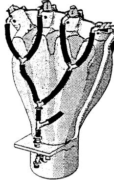
The majority of nozzles for mistblowers are made of ceramic material. This ensures long life even at high working pressures but even so they do wear. If nozzle output is more than 10 % in relation to the theoretical (table) value, the nozzle should be replaced.
