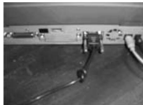
The communication cable with the "Hardware Halt" is plugged into the JobCom.
