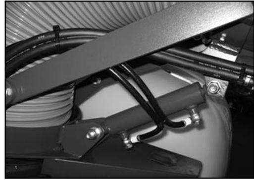
For a  $180^{\circ}$  rotation, another double acting outlet is necessary. This movement enables you to carry out the treatment on one side or the other of the CANNON, regardless of the direction the tractor is going.
