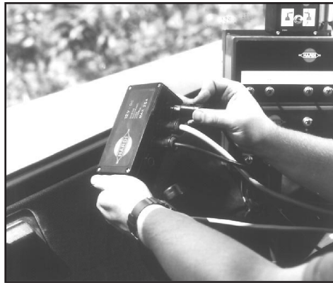
Fig. 16 (12-volt junction box for 12-volt hook-up for ESC controls, foam marker, boom hydraulic controls, etc)
