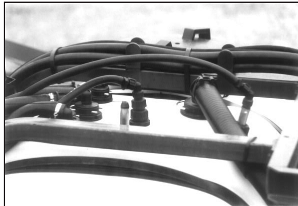
Fig. 56 Rinse Nozzle on Top of Tank
