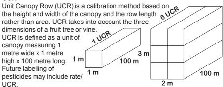
The Controller can be set up for mistblower to handle UCR. This is done from the extended menu. See "Extended menu" or contact your HARDI service centre if the Controller is not set up for UCR.
