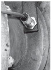
A speed/switch harness (**A**) and extension cable are needed to connect the speed transducer to the Controller.
