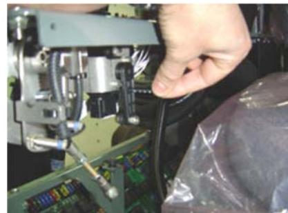
3. Adjust the threaded rod between the joystick and the potentiometer and tighten the two jamb nuts on the ball joints.
