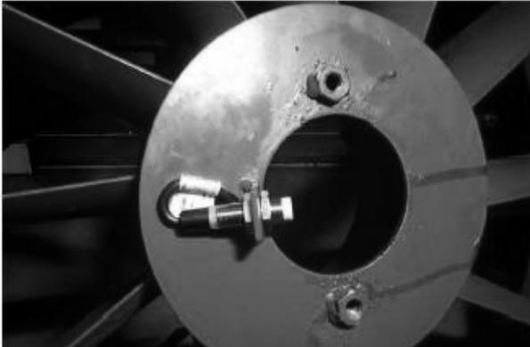
**Picture 7 Fan speed sensor**
