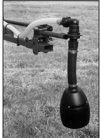
The Foam Marker helps prevent skipping or over lapping during spray application of spray solution, both which can be costly. HARDI® Foam Marker features a trailer mounted compressor, poly tank, extruded foamer hoses and in-cab electrical controls providing right or left drop selection and the rate/quality of foam droplets. Refer to the Foam Marker Operator's Manual for complete operation instructions.
