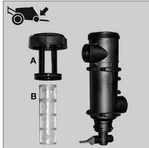
**⚠ DANGER!** Before opening the Cyclone filter, the Suction SmartValve must always be turned to the unused position and the pressure SmartValve to "Main tank" (both levers pointing forward)! If not, spraying liquid can hit you when opening the filter, and drain from the tank!
