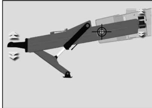
For transport, raise the support leg all the way up and turn the hydraulic valve to the “locked” position.
