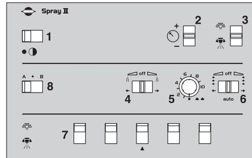
In order to close the entire boom, switch ON/OFF (3) to OFF position. This returns the pump output to the tank through the return system. The diaphragm Non-drip valves ensure instantaneous closing of all nozzles.
