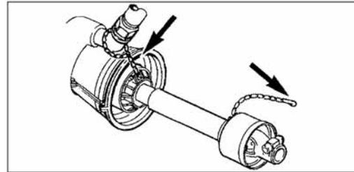
8. To ensure long life of the transmission shaft, try to avoid working angles greater than 15°.
