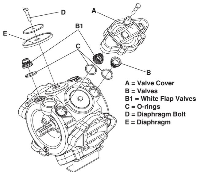
Diaphragm pump overhaul kit (valves, seals, diaphragms, etc.)
