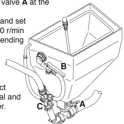
**Note:** The measuring scale in the hopper can only be used if the sprayer is parked on level ground! It is recommended to use a measuring jug for best accuracy.
