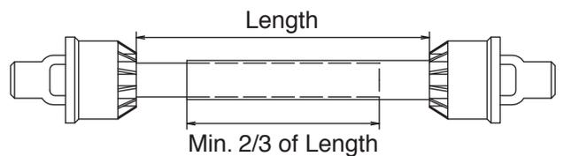
4. The two parts are shortened equally. Use a saw, and file the profiles afterwards to remove burrs.
