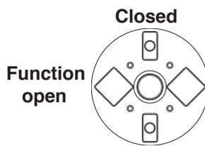
Decals are fitted to the faces of the 3-way valves indicating the direction of flow of the liquid.
