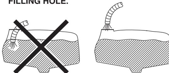
**IF THE HOSE IS LEAD TO THE BOTTOM OF THE TANK, AND THE WATER PUMP AT THE WATER SUPPLY PLANT STOPS, CHEMICALS CAN BE SIPHONED BACK AND CONTAMINATE THE WATER SUPPLY LINES.**
