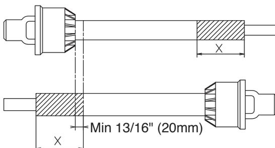
**Note:** The minimum allowable overlap for the shaft depends on the pump model.
