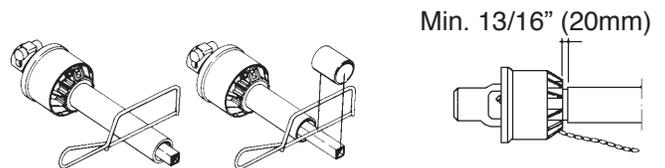
5. Grease the profiles, and assemble male and female parts again.
