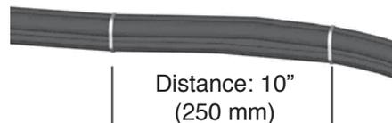
The hoses must be secured with tie straps at 10" (250 mm) spacing between MANIFOLD valves and front tank.
