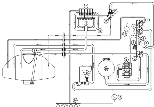
1. Empty the sprayer as much as possible. Turn off self-cleaning filter return valve **12** (diaphragm system only) and air bleed-off valve **5** and spray until air comes out of all nozzles.
