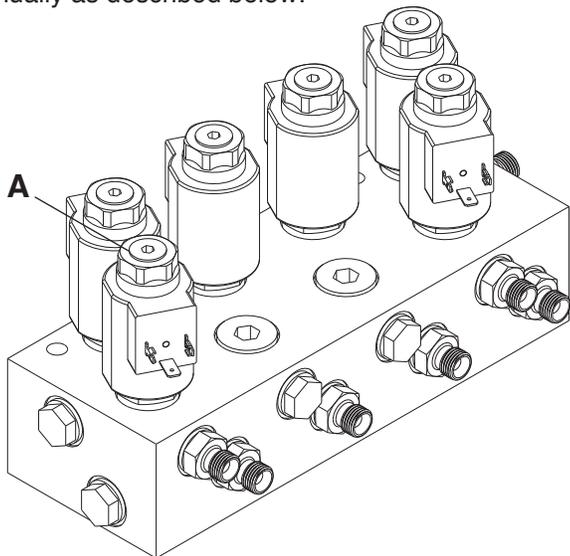
1. Unscrew top part **A** from solenoid valve. Notice the small pin in the hollow of the valve.
