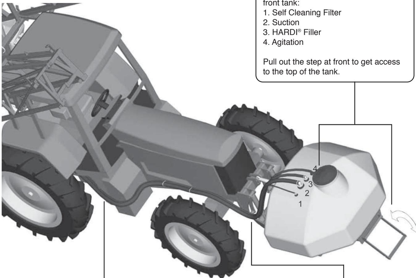
Attach the hoses with fittings to the front tank:
