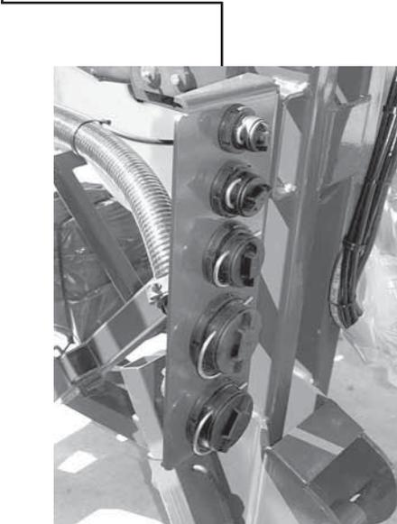
3. Fasten the fittings/hoses to the mounting on the DELTA.
