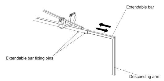
The position of the descending arm can be regulated with regards to width, in order to adapt the machine to match the row spacing. Once the required position has been chosen, locking bolts are employed to prevent any movement of the bar.
