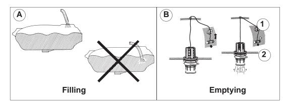
To empty the tank with the drain valve, pull the red handle located on the upper right-hand side. The valve is spring-loaded to return it to the closed position, but can be kept open by pulling the string out and upwards into the V-shaped slot 1. To close the drain valve again, pull the red handle down and release (2). The valve will close automatically (B).
