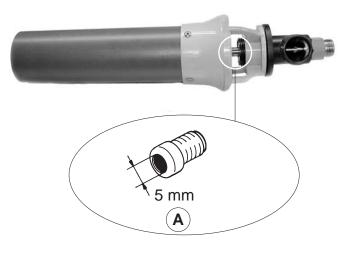
The restrictor should be replaced in the following way:
