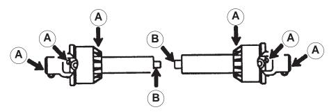
**NOTE.** In all the HARDI<sup>®</sup> ARROW models, the P.T.O. shaft that connects the pump to the fan must also be greased.
