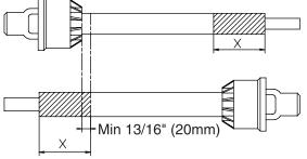
**Note:** The shaft must always have a minimum overlap of 1/3 the length.
