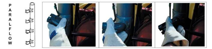
The height of the spout assembly can also be adjusted, and the width adapted to suit the row spacing. Loosen the nut (S) and move the bracket up or down. In order to alter the width, loosen the two r(T).
