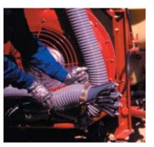
The pneumatic paraflow model's spouts can also be individually adjusted to point towards the areas that you wish to spray.
