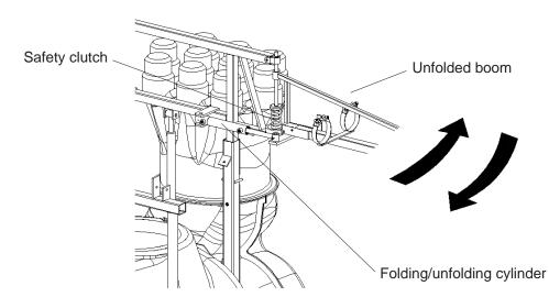
The folding/unfolding cylinder enables the boom to be placed in the unfolded (working) position or in the folded (transport) position.
