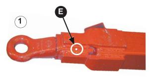
The turnable hitch drawbar (2) has two grease nipples, (E) and (F).
