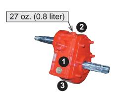
The oil fill is at the top of the mechanism, behind the tank.
