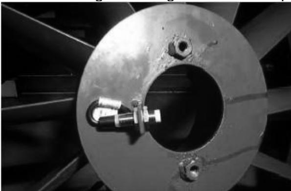
**Picture 6 Fan speed sensor**
