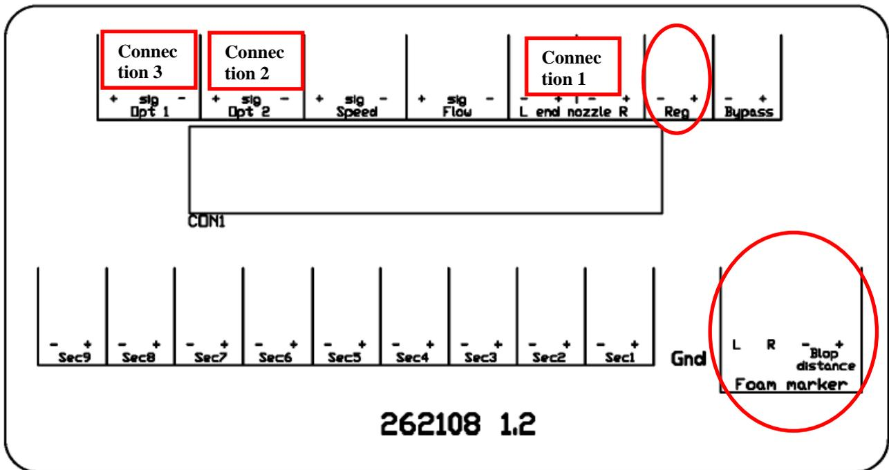
Picture 14 PCB for sections valves (9 section's PCB)
