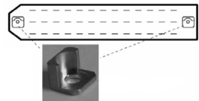
The dowel is set as when viewed into the plug on the cable. Re-coding the dowel allows switching from liquid to hydraulic and vice-versa.
