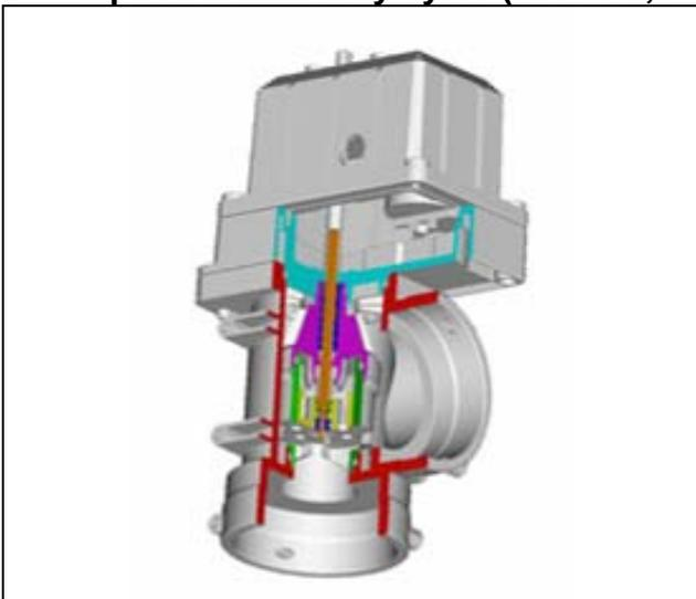
Figure 3 Pressure regulation valve
