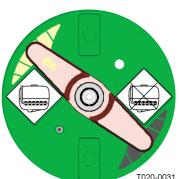
Handle is positioned near the tip of the arrow (in agitation side of the disk). Agitation quantity is 10%.
