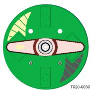
Handle is positioned at the middle of the arrow (in agitation side of the disk). Agitation quantity is 50%.
