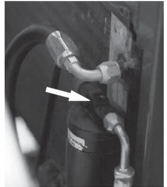
**WARNING!** Air conditioning circuit contains FREON 12 under pressure. Change of e.g. hoses, requires the circuit to be depressurized first and drained for freon. Do not try to repair air conditioning yourself - repairs require a skilled technician and special equipment.
