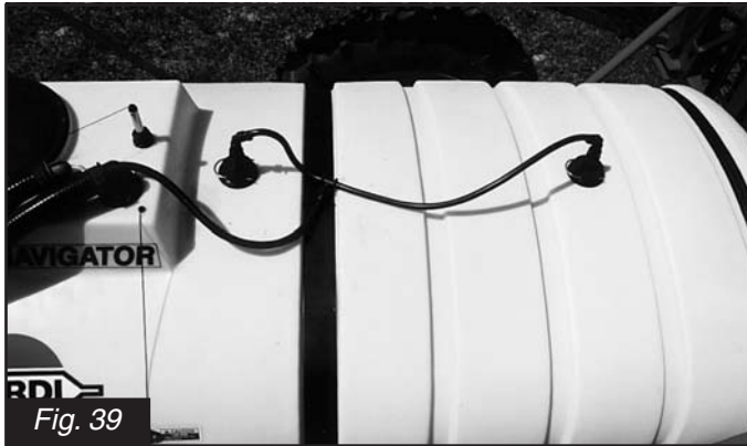
Rinse Nozzle on Top of Tank
