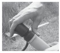
When the battery pack is assembled, observe that the O-rings are placed in a correct way. Otherwise, water will penetrate the battery compartment resulting in irreversible damage.
