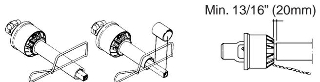
5. Grease the profiles, and assemble male and female parts again.
