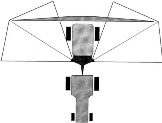
The 2 boom light lamps **A** are mounted to the railing of the platform (one at each side) and are positioned to illuminate both boom wings.
