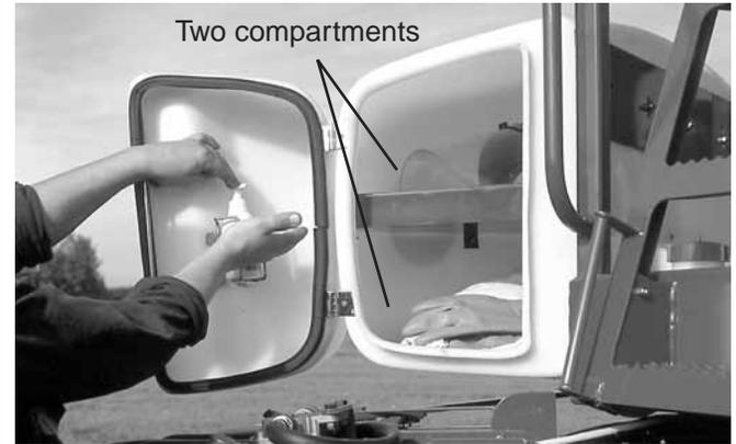
A soap dispenser can be fitted in a device on the inside of the locker door.
