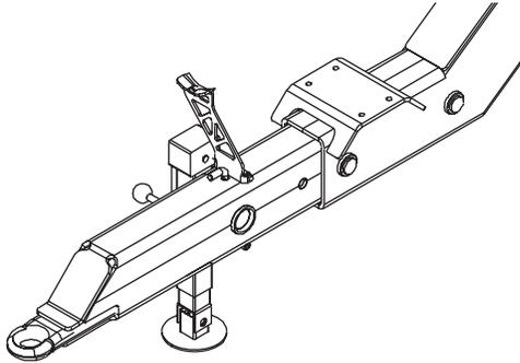
The support leg is stored in the storage bracket on the right side of the trailer when the sprayer is attached to the tractor. To remove the support leg: Lift the leg, remove the pin and pull out the support leg.
