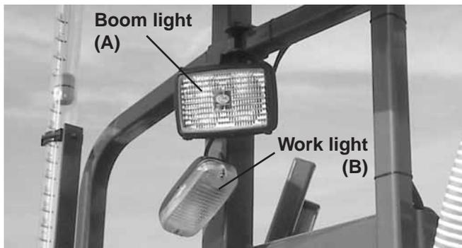
The work light lamp **B** is also mounted to the railing of the platform above the MANIFOLD valves. This lamp is positioned to illuminate the HARDI® FILLER and the SMART VALVE system.
