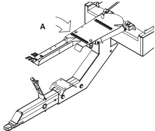
Check that the length of the hoses and cables is sufficient in tight turns, especially when the optional steering drawbar is fitted.
