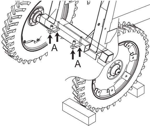
3. Place wheel stops in front of and behind the RH wheel. Jack up the LH wheel, support and secure the sprayer frame.
