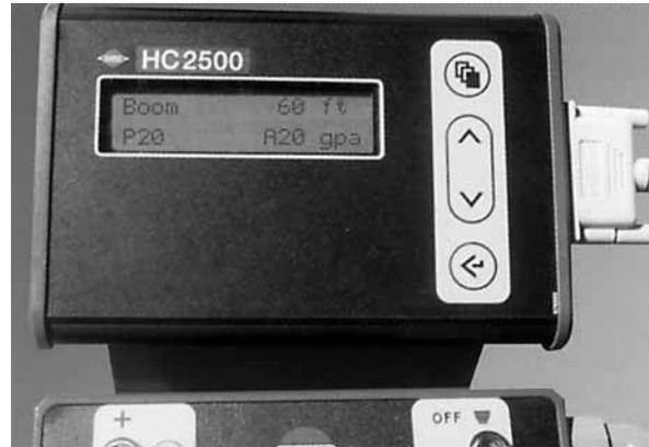
The HARDI® Controller 2500 permits automatic control of the application rate. This allows you to concentrate on driving as the rate is automatically maintained by the HC 2500. Press the "up" or "down" arrow keys to change the application rate. Easy, quick and simple. Up to 8 spray boom section control is possible.
