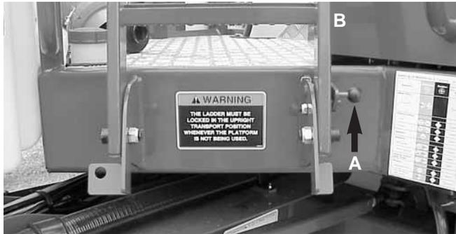
**Down:** Lift the red knob **A** to disengage the locking device and swing the ladder **B** down.
