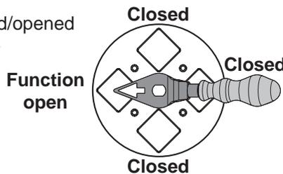
Symbols (shown below) are fitted to the faces of the manifold valves indicating direction of flow of the liquid.
