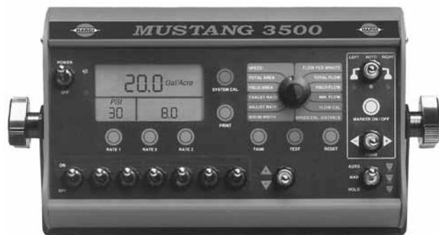
The Mustang 3500 Controller offers fully integrated boom controls (3 - 7 sections), integrated foam marker controls, integrated TWIN FORCE controls, 3 possible preprogrammed application rate settings, 9 different field counters, DGPS compatible, prepared for communication with Precision Farming Terminals and pocket PC's (iPAQ - models: 3650, 3670), variable rate application, rain & dust proof and 3 year warranty.
