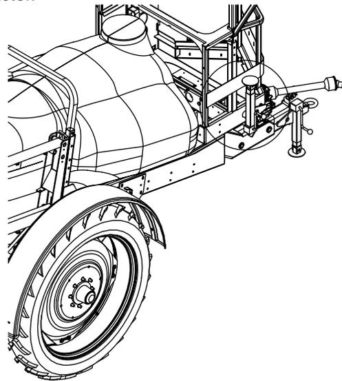
To remove the support jack from the drawbar hitch: Lift the leg, remove the linch pin and pull out the support jack. The support jack can then be mounted to the storage bracket and secured by the linch pin.
