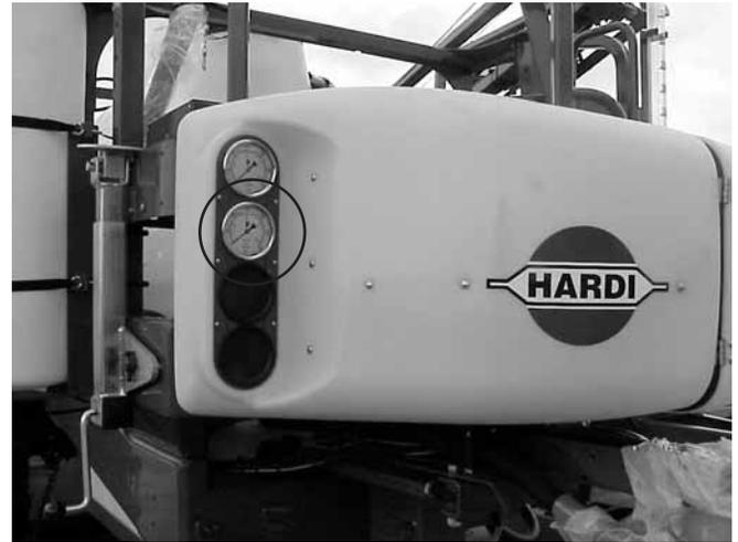
Boom Pressure and Manifold Pressure Gauges
