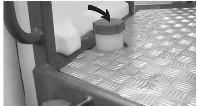
The water from this tank is for hand washing, cleaning of clogged nozzles etc. The valve is located within reach from the SMART VALVES and is opened/closed by a valve handle.
