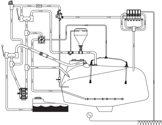
1. Empty the sprayer as much as possible. Turn the top green pressure valve towards "No Agitation" and spray until air comes out of all nozzles.
