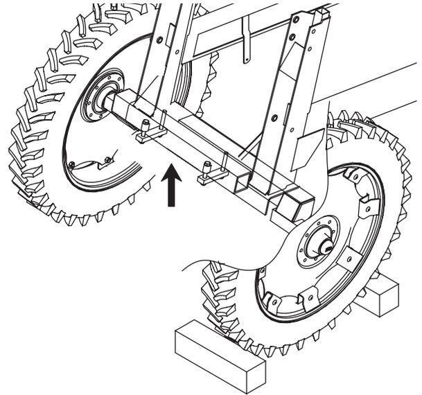
**IMPORTANT!** Place the jack under the axle and lift the wheel to remove any load from the axle clamps before tightening the axle clamp bolts to the specified torque.
