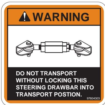
When the hydraulic steering is needed again, remove the front pin and snap ring, swing the transport lock out to the field position and secure with pin and snap ring.
