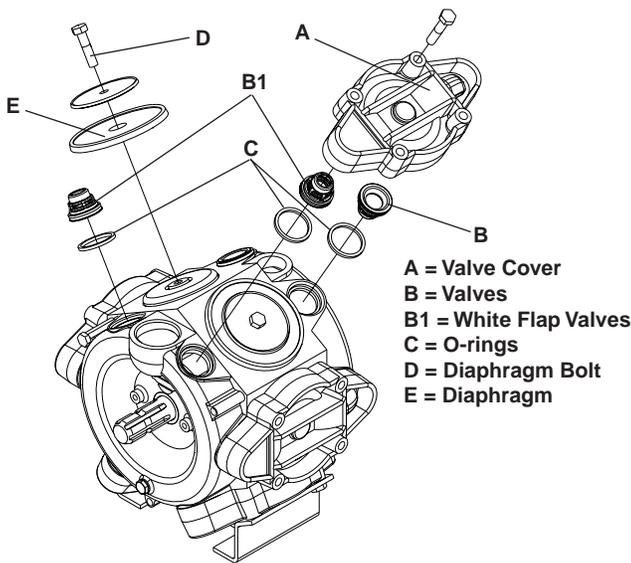
Diaphragm pump overhaul kit (valves, seals, diaphragms, etc.)
