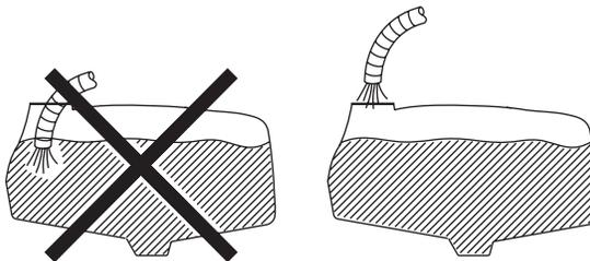
**IF THE HOSE IS LEAD TO THE BOTTOM OF THE TANK, AND THE WATER PUMP AT THE WATER SUPPLY PLANT STOPS, CHEMICALS CAN BE SIPHONED BACK AND CONTAMINATE THE WATER SUPPLY LINES.**
