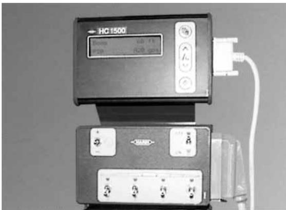
The HARDI® Monitor 1500 monitors the application rate. When used with the electric control unit switch box, correct area covered and up to 8 spray boom section control is possible.
