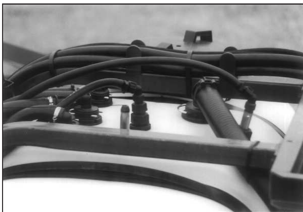
Fig. 61 Rinse Nozzle on Top of Tank
