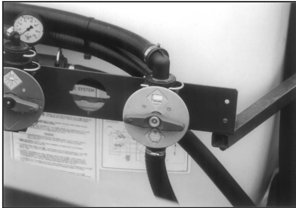
Fig. 67 Agitation Bypass Valve
