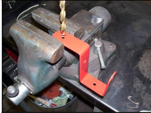
**Figure 10: Drilling the main lift sensor bracket**
