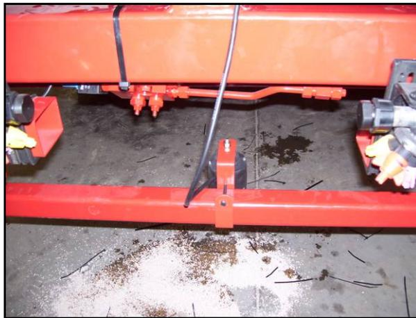
**Figure 11: Main Lift Sensor Installed**
