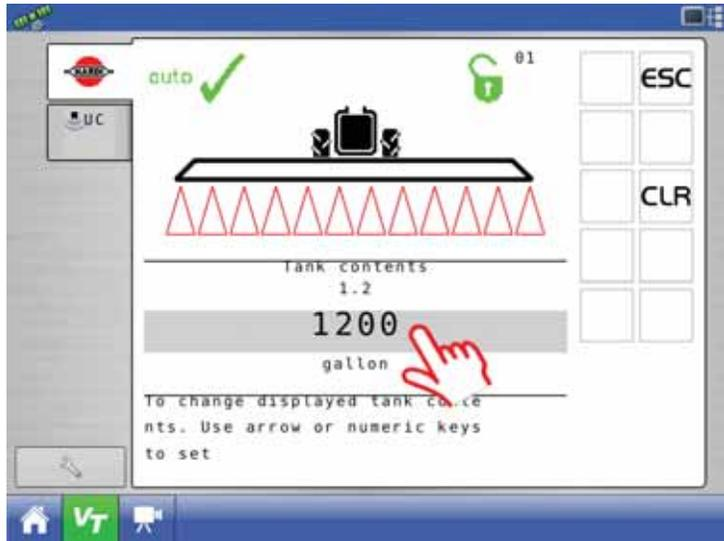
5. Enter the new tank contents value on the numeric key pad and select check mark to confirm.
