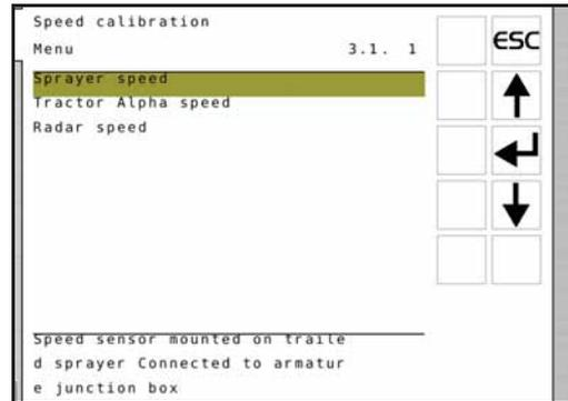
It is possible to calibrate the speed sensor in different ways. You may enter a theoretical speed constant or perform a practical calibration.
