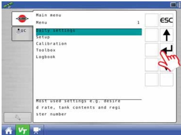
3. Scroll to "Tank contents" with {up} or {down} arrows and select enter to confirm.
