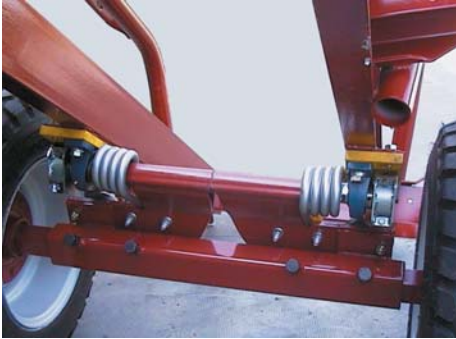
Suspension kit is added to the housing.
