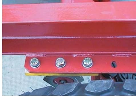
Anchored to the frame by three bolts.
