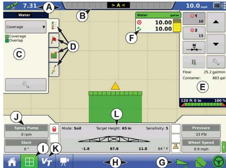
The task bar (H) displays buttons relating to various functions of the display. These buttons and status indicators include:
