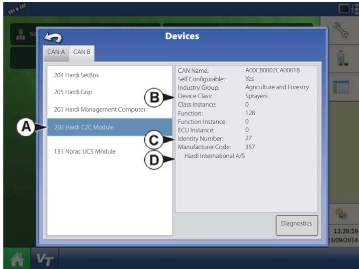
Pressing the Diagnostics button on the Devices screen brings up the ISO Node Diagnostics screen which shows the following information.
