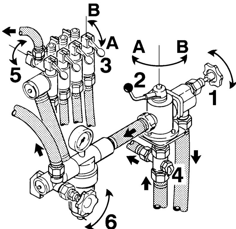
1. Open or close lever 4 depending on whether pressure agitation is required. (Remember pressure agitation takes 5% to 10% of pump output).
