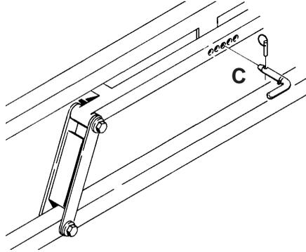
**For HB boom** - Under normal conditions the trapeze is always active. When spraying on flat fields, use pos. 2. On sloping terrain the boom can be slanted (pos. 1 or 3) and still maintain an active trapeze.
