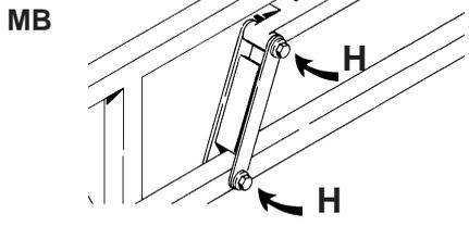
Wire tension - **HB boom** only. Slack wires result in excessive boom yawn. To adjust, loosen rigging screw lock nuts and turn. If overtightened it will not be possible to fold arm down.
