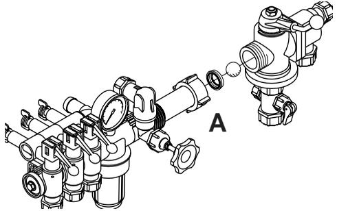
Check the ball for sharp edges and scratches and check the ball seat for cracks and wear - replace if necessary.
