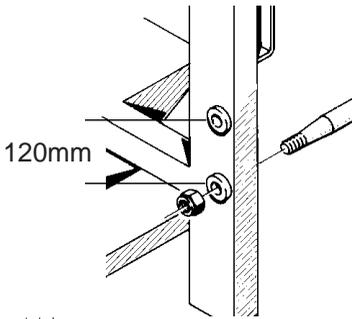
For **HB boom** - For increased stability when the sprayer is detached, retractable supports are located under the frame. Extend before detaching. Retract after attached.
