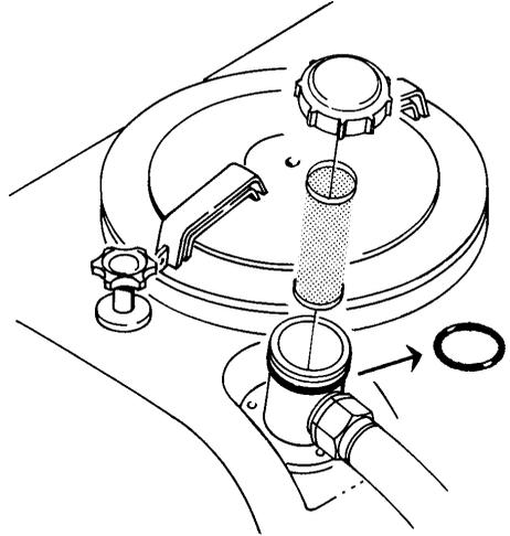
The main filter protecting sprayer components is the suction filter at the top of the tank. Check it regularly.
