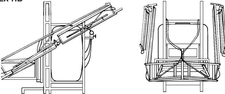
The **MB** spray boom (10 or 12 metre) or the **HB** spray boom (12, 15, 16 or 18 metre) is fitted. The boom is supported by a trapeze which protects the boom against vibrations and shocks when driving on uneven ground. This ensures longer boom life and improves boom stability for an optimal spray pattern. Height adjustment of the boom is hydraulic. The boom is fitted with spring loaded breakaways at the pivots.
