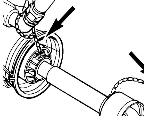
To ensure long life of the transmission shaft, try to avoid working angles greater than 15°.
