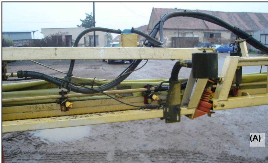
Figure 11 - Suggested Bracket Mounting Location (viewed from front) on 36m HAZ
