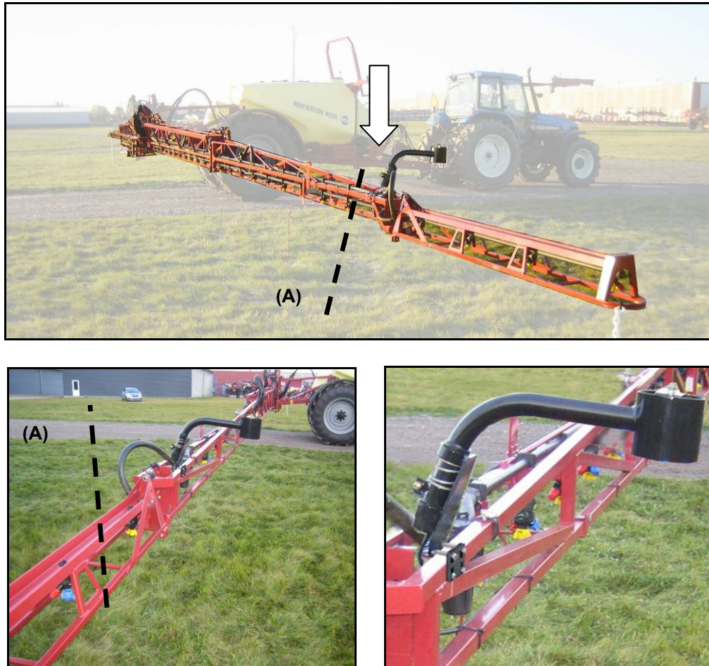
Figure 12 - Suggested Bracket Mounting Location on LPZ Boom
