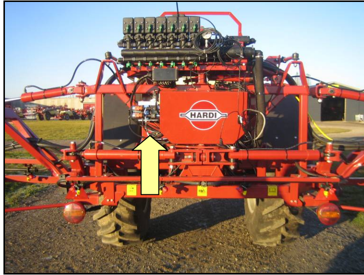
Figure 30 – Valve Block Mounting Location on LPZ
