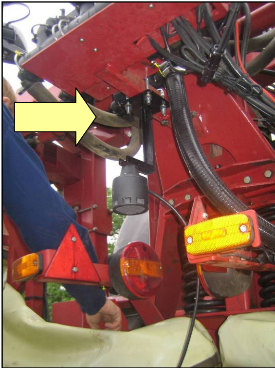
Figure 13: Main Lift Sensor Mounted to the HPZ/HAZ Center Part
