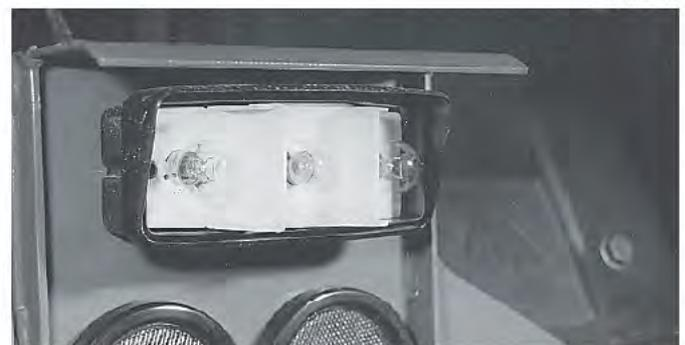
**Front position lamp and direction indicator bulb**
