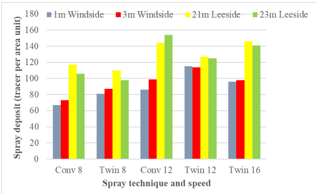
Figure 2. Deposition below the boom in different distances from the end of the boom. The wind direction was perpendicular to driving direction with petri dishes placed 1 and 3 m from the end of the boom in the wind side (1m W and 3m W) and placed 3 and 1 m from the end of the boom in the lee side (21m L and 23m L). Test at high wind speed May 2018
