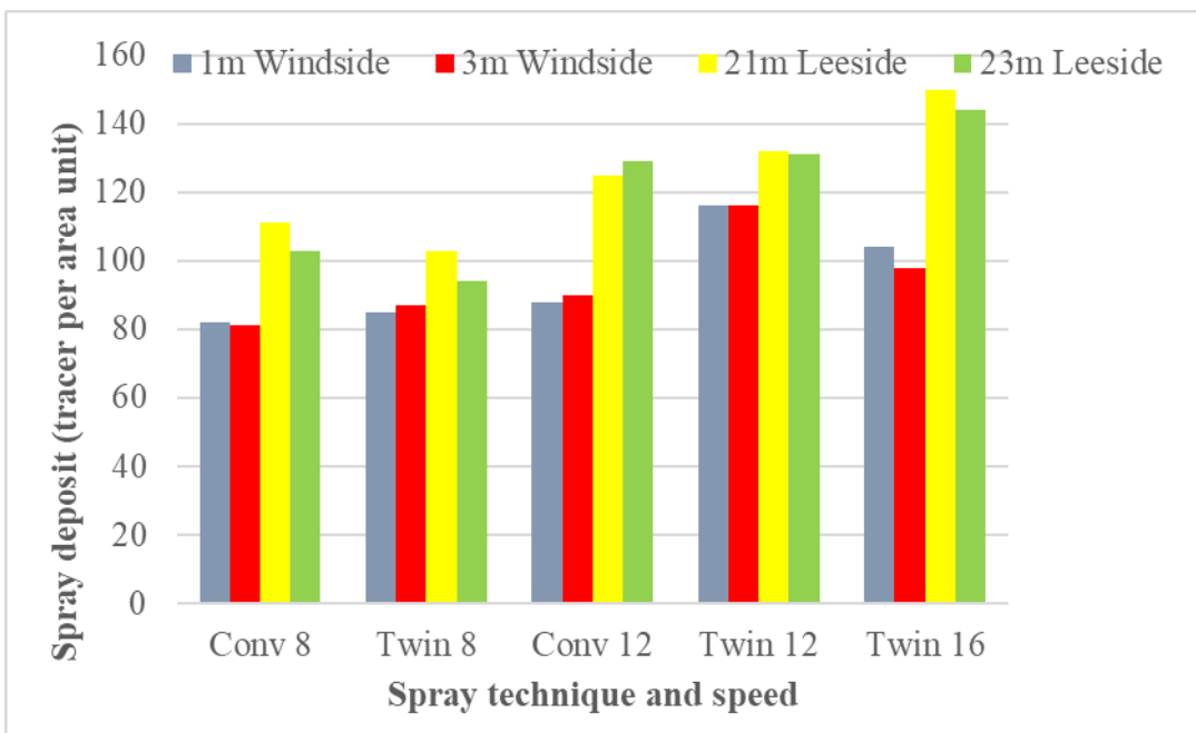
Figure 3. Deposition below the boom in different distances from the end of the boom. The wind direction was perpendicular to driving direction with petri dishes placed 1 and 3 m from the end of the boom in the wind side (1m W and 3m W) and placed 3 and 1 m from the end of the boom in the lee side (21m L and 23m L). Mean of tests at low/normal and high wind speed 2017 & 2018.
